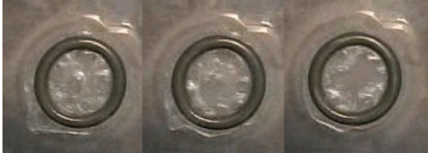
Fig. 12.14 Traveling and decaying of cnoidal waves on the external surface taken at three different moments of time
