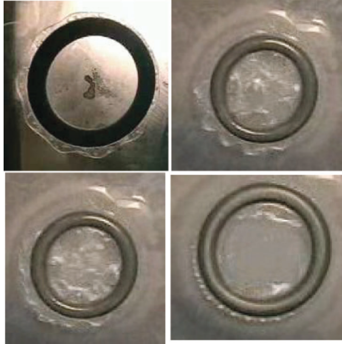
Fig. 12.12 Surface waves in a two-dimensional shallow circular layer of liquid nitrogen around a rigid core. Modes with l = 12 –30 and amplitude in the range 1–5 mm can be measured, depending on the depth of the layer. The waves travel with a circular speed of 20 – 40 \text{ cm s}^{-1} . In the figure the core has a diameter of 3 cm
